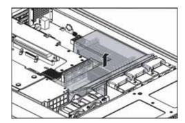
4 Lift the release tab (1) (similar on both fan cages), then push the fan cage in the direction of the arrow (2) to unlock it from the chassis.
